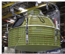
Artemis IV Capsule Pressure Vessel Welding Complete
