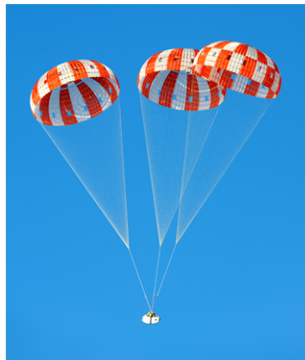
Orion Capsule Parachute Testing
